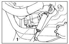
1. Engine oil drain bolt
